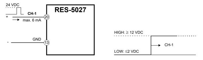
Activation of the CH-1 signal is not accepted during performance of the AUTOCAL function or with an active RESET signal.
