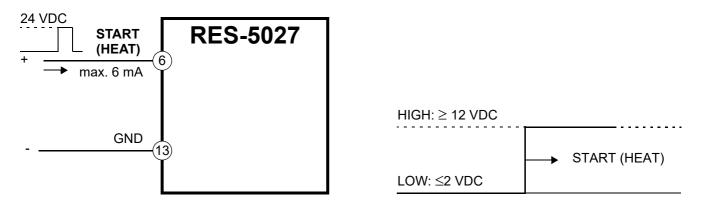
During execution of the AUTOCAL function or when the RESET signal is active, activation of the START signal is not accepted.
