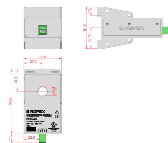
Mounting on DIN-rail  $35 \times 7.5$  mm or  $35 \times 15$  mm (EN 60715). If the high-current wire cannot be routed through the opening provided, an HCB-1 high-current rail must be used.
