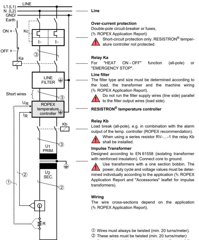
if several control loops are laid together ("crosstalk"). ③ Twisting (min. 20 turns/meter) is recommended to improve EMC.
