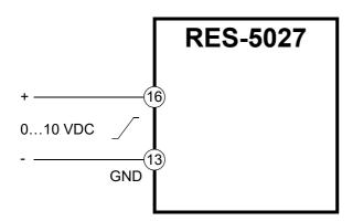
The correlation between the applied voltage and the ACTUAL temperature is linear.
