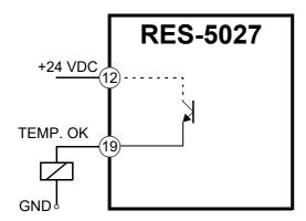
While the constant power setting mode is active ( section 8.7 "CH-1 signal" on page 26) this output remains inactive.
