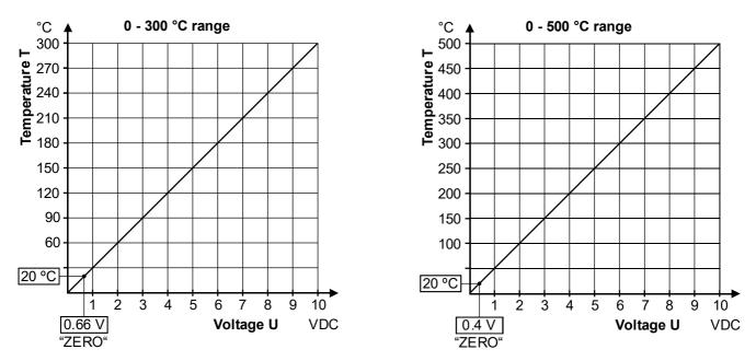
The correlation between the change in the output voltage and the ACTUAL temperature is linear.
