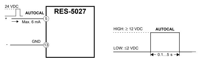
The automatic calibration process lasts about 10...15 seconds. The heating element is not additionally heated during this process.
