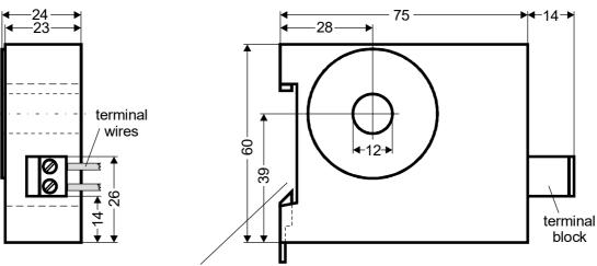
Snap-on for DIN-rail 35 x 7,5 mm or 35 x 15 mm (EN 60715)
