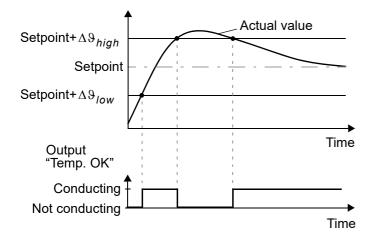
As soon as the ACTUAL temperature is again within the specified tolerance band, the output signal is switched back on again.
