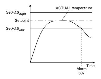
If the temperature diagnosis has not switched on before the START signal is deactivated (i.e. The ACTUAL temperature has not exceeded the lower tolerance band limit or dropped below the upper tolerance band limit), the related error no. 309, 310 is output and the alarm relay switches on.
