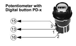
To be able to specify the setpoint with a potentiometer, the controller provides a reference voltage of +10 VDC (±5%) at terminal 15.
