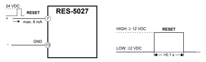
During activation of the RESET signal, the actual value output goes to 0...3 °C (i.e. approx. 0 VDC). This can be evaluated as feedback by the higher-level controller (e.g. PLC).
