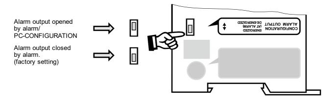
When the "Alarm output opens with Alarm/PC CONFIGURATION" is selected, additional configurations for the behaviour of the alarm output can be set through the ROPEX visualisation software ( $\$  section 8.17 "USB interface for visualisation software ROPEXvisual<sup>®</sup>" on page 35).
