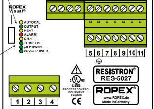
The LEDs display additional operating statuses of the controller besides the functions in the above illustration. These are shown in detail in the following table:
