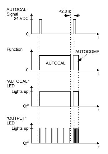
During execution of the AUTOCOMP function, the "OUTPUT" LED flashes several times and the actual value output (terminal 17+13) goes to 0...3 °C (i.e. approx. 0 VDC).
